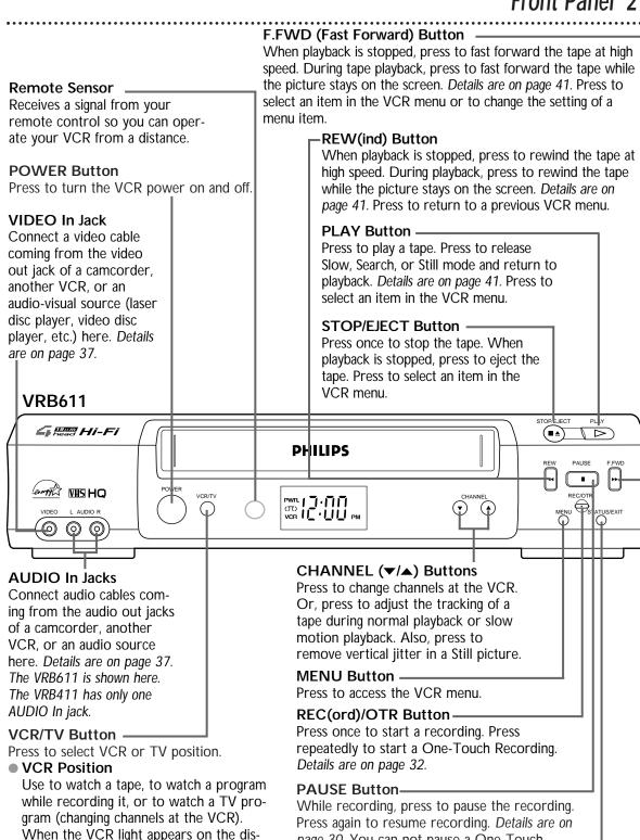
Press again to resume recording. *Details are on page 30.* You can not pause a One-Touch Recording. During tape playback, press to freeze the picture. Press again to resume playback. *Details are on page 41.*
